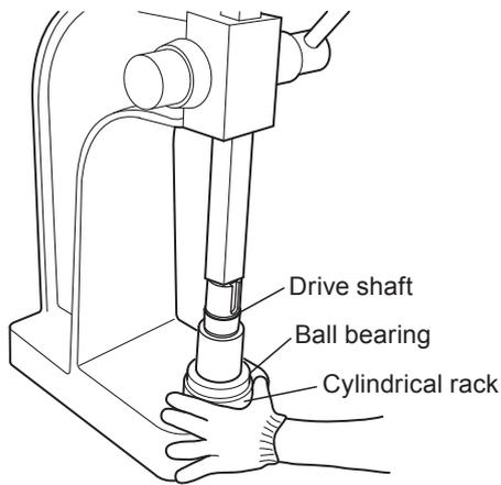
2. Place the bearing spacer on the ball bearing along with its circumference. And then press-fit the other ball bearing into the shaft.
