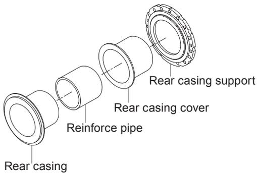
10. Remove the rear casing cover and the rear casing. Be careful not to scratch a sealing surface on the rear casing.
