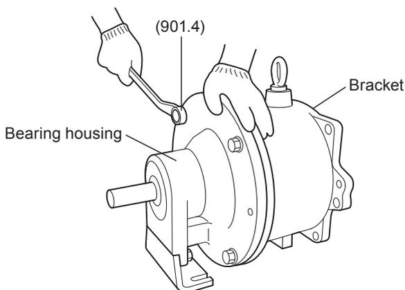
9. Place the bracket and bearing housing on the level and fix them with hex head bolts (901.4).
