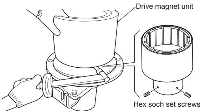
7. Unscrew the hex socket set screws (908.1) once and apply the LOCKTITE to threads. And then screw them to fix the drive magnet unit by the tightening torque below.
