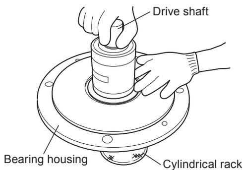
4. Mount the drive shaft assembly into the bearing housing.
