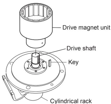
6. Fit the key onto the drive shaft and then mount the drive magnet unit.
