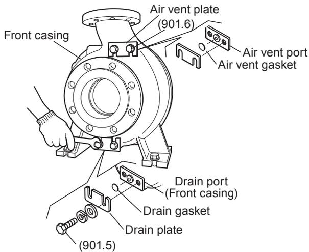
12. Place an air vent gasket and air vent plate on the air vent port which is positioned on top of the front casing. And fix them with the hex head bolts (901.6) Place a drain gasket and drain plate on the drain port which is positioned at the bottom of the front casing. And fix them with the hex head bolts (901.5).
