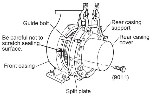
14. Crane and mount the split plate assembly into the front casing and then fix it with hex head bolts (901.1). Install guide bolts to both sides of the front casing for easy mounting. Do not hit the impeller unit onto the front casing when not using guide bolts.
