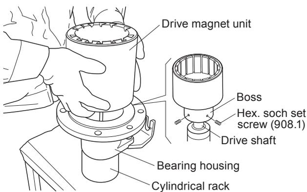
2. Loosen the hex soch set screws (908.1) and remove the drive magnet unit from the drive shaft. Then remove a key from the shaft.
