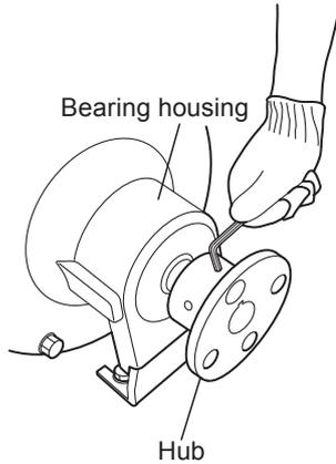
5. Pull out the drive shaft along with the ball bearing from the bearing housing.
