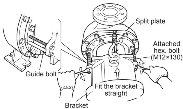
16. Remove the guide bolts and install them on the rear casing support. Take the attached two hexagon bolts (M12×130) and screw them into both upper holes on the bracket edges all the way. Using guide bolts, the bracket can be mounted straight without hitting against the rear casing cover.
