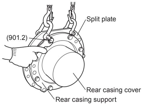
9. Remove the hex head bolts (901.2) and remove the rear casing support.
