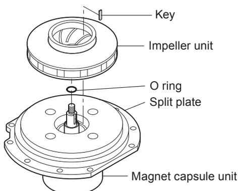
4. Insert the impeller unit to the shaft, mating the key groove.
