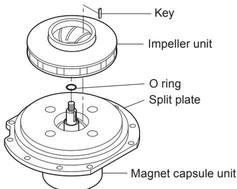
12. Pull the impeller unit out of the split plate. Jiggle the impeller unit as necessary.
