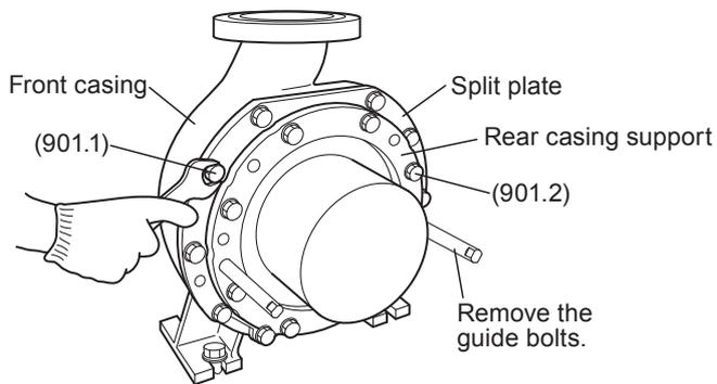
15. Tighten the rear casing support fixing bolts (901.2) and split plate assembly fixing bolts (901.1) at the tightening torque below.
