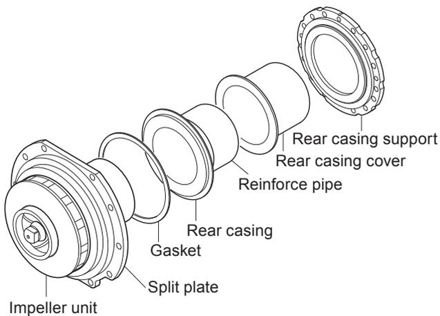
9. Remove foreign matters from the magnet capsule unit. Then place the gasket in the split plate. And then fit the rear casing and the rear casing cover.
