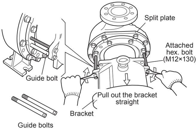
5. Screw the guide bolts into the rear casing support via both bottom holes on the bracket edges.
