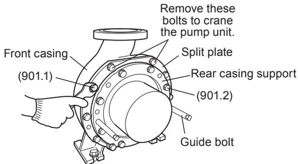
7. Unscrew guide bolts from the rear casing support. And then screw the bolts into the front casing through the split plate.
