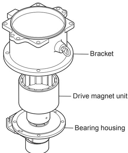
8. Place the bracket to the bearing housing.
