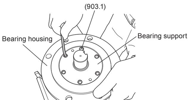
3. Remove the hex. soch head bolts (903.1) and detach the bearing cover.
