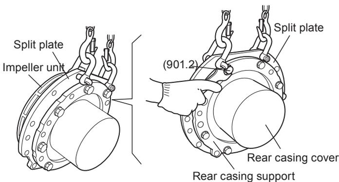
10. Hold up the split plate with the crane for the impeller unit not to be pressed onto a floor. Then temporary mount the rear casing with the hex. head bolts (901.2).
