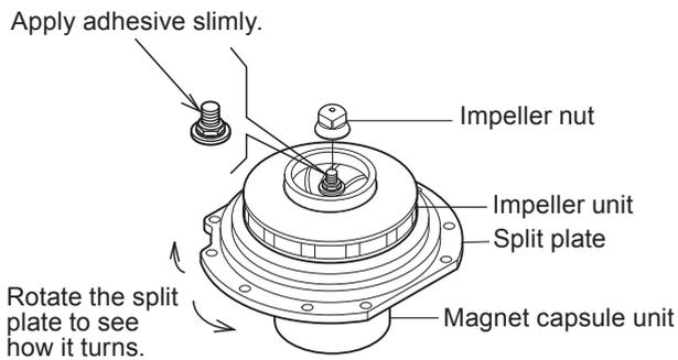
8. Tighten the impeller nut while holding the impeller unit. Apply adhesive slimly on the threads of the shaft not to allow the nut to loosen.
