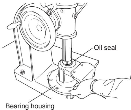
3. Use a hand press to press-fit the oil seal into the groove on the bearing housing via a plastic bar.
