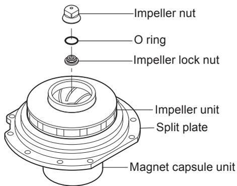
11. Remove the impeller nut and the impeller lock nut.
