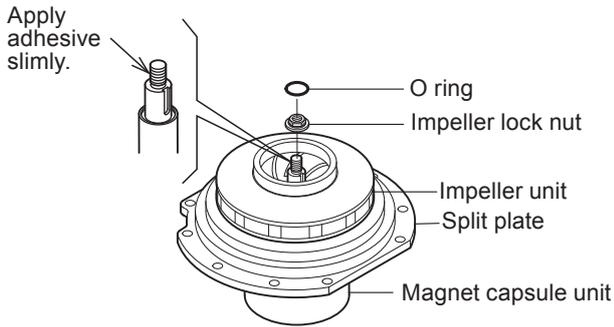
6. Fit the O ring into the groove on the impeller unit in place.
