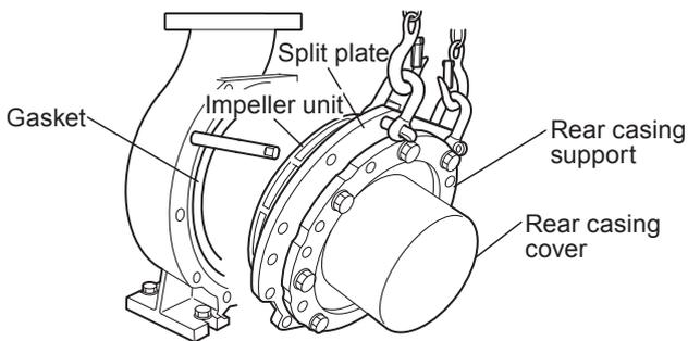
13. Place the gasket in the front casing. If the gasket can't stay in the groove on the front casing, slimly apply fluorine grease so that the gasket can't come off.
