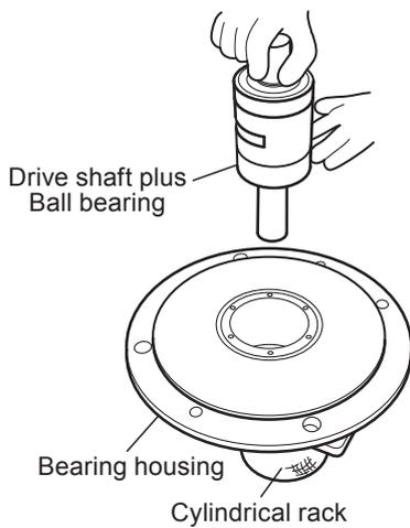
6. Remove the ball bearing and the bearing spacer from the drive shaft.
