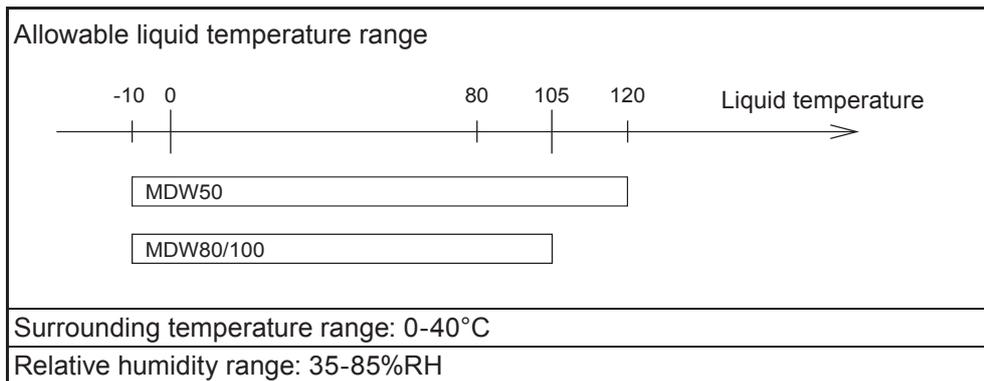
\*Note that viscosity, vapour pressure or corrosiveness changes with liquid temperature. The change is shown in performance such as flow rate while the pump itself is not affected.
