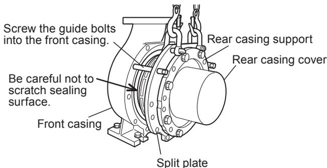
8. Crane the split plate with accompanying parts to separate them from the front casing.
