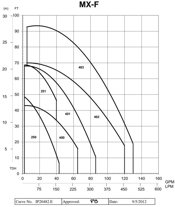
Performance based on water at 70°F (21°C). Fluids with specific gravities other than 1.0 should be reviewed by the
