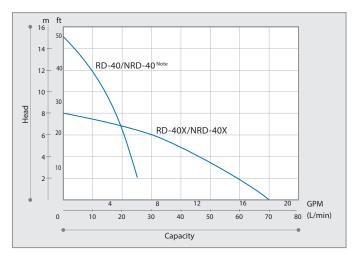
Note: Do not exceed 6.6 GPM in operation, or cavitation may take place. The above curves are based on operation with a 5V external control signal.
