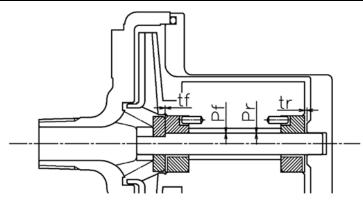
·Clearance between Impeller and casing
