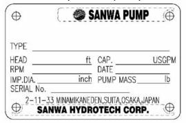
TYPE: Pump model and pump code
