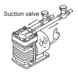
• The APN-S110 is designed for vacuum application only. Do not pressurize the discharge line of the pump.
