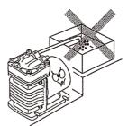
Use care handling the pump. Do not drop. An impact may affect pump performance. Do not use a pump that has been damaged to avoid the risk of electrical damage or shock.
